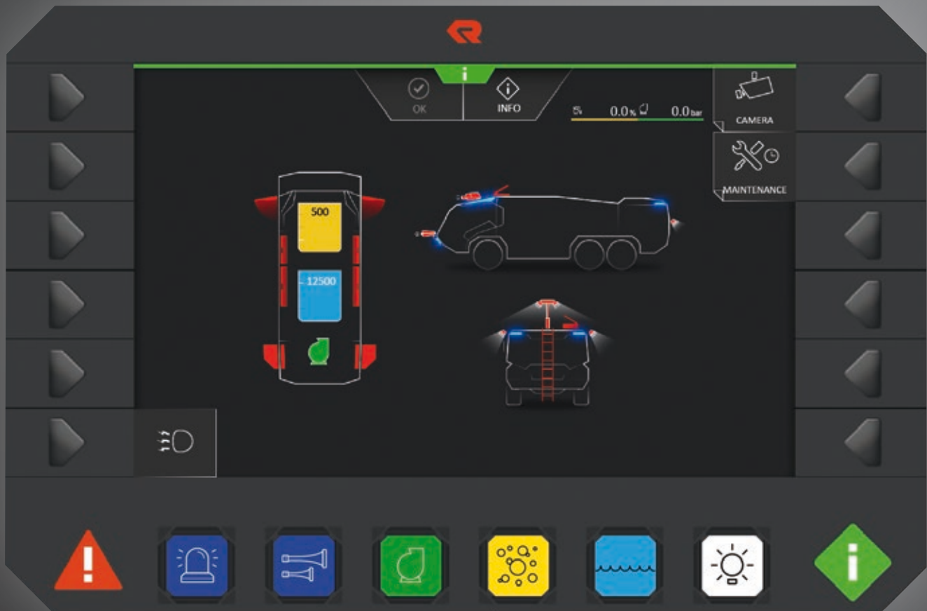
10" RBC LCS display: HD resolution, touch function, and automatic color switching adapted to the ambient conditions.
