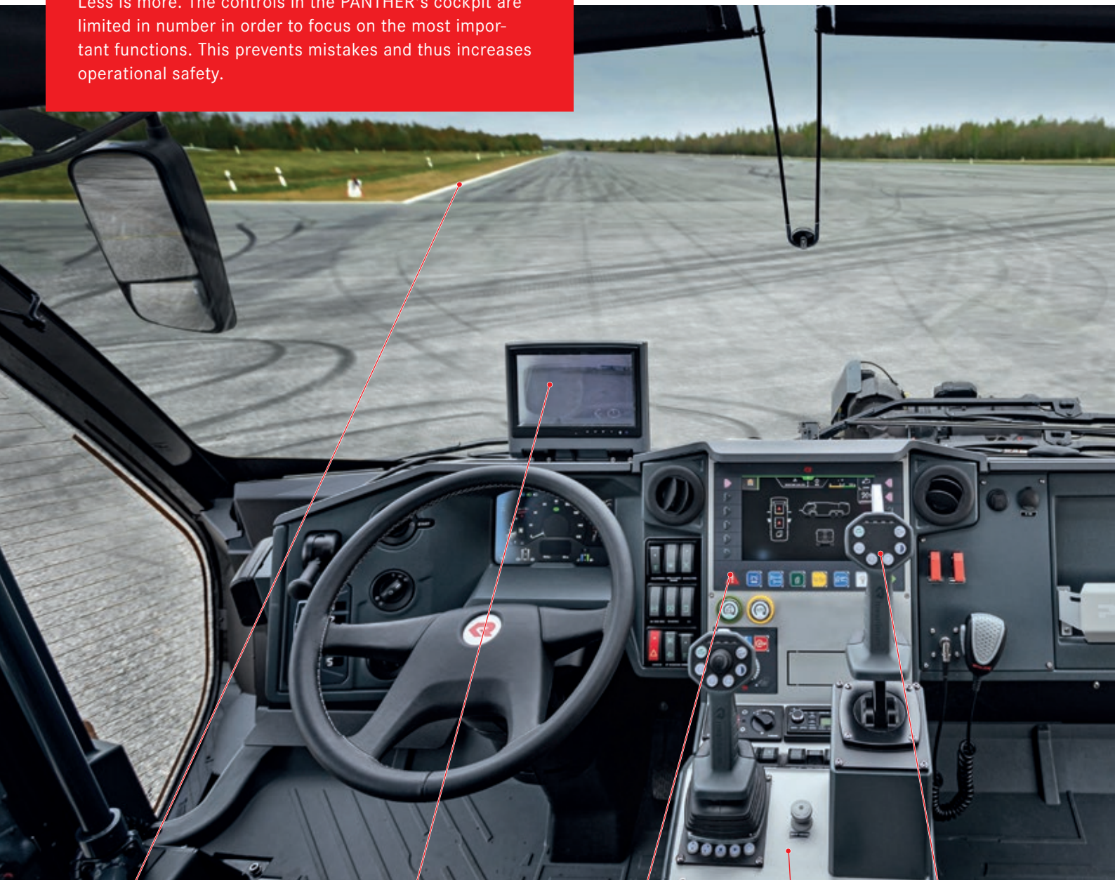
Larger visual field thanks to optimized A-column and control panel
