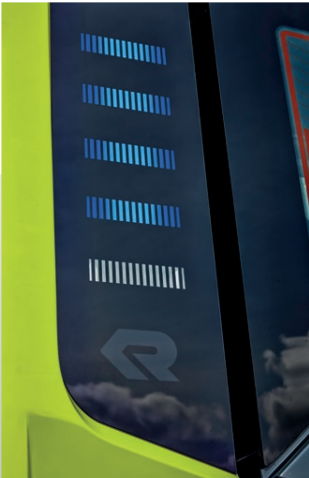
External tank indicator
