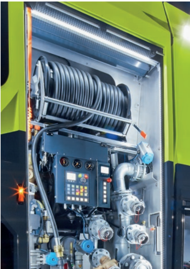
Pump room illumination
