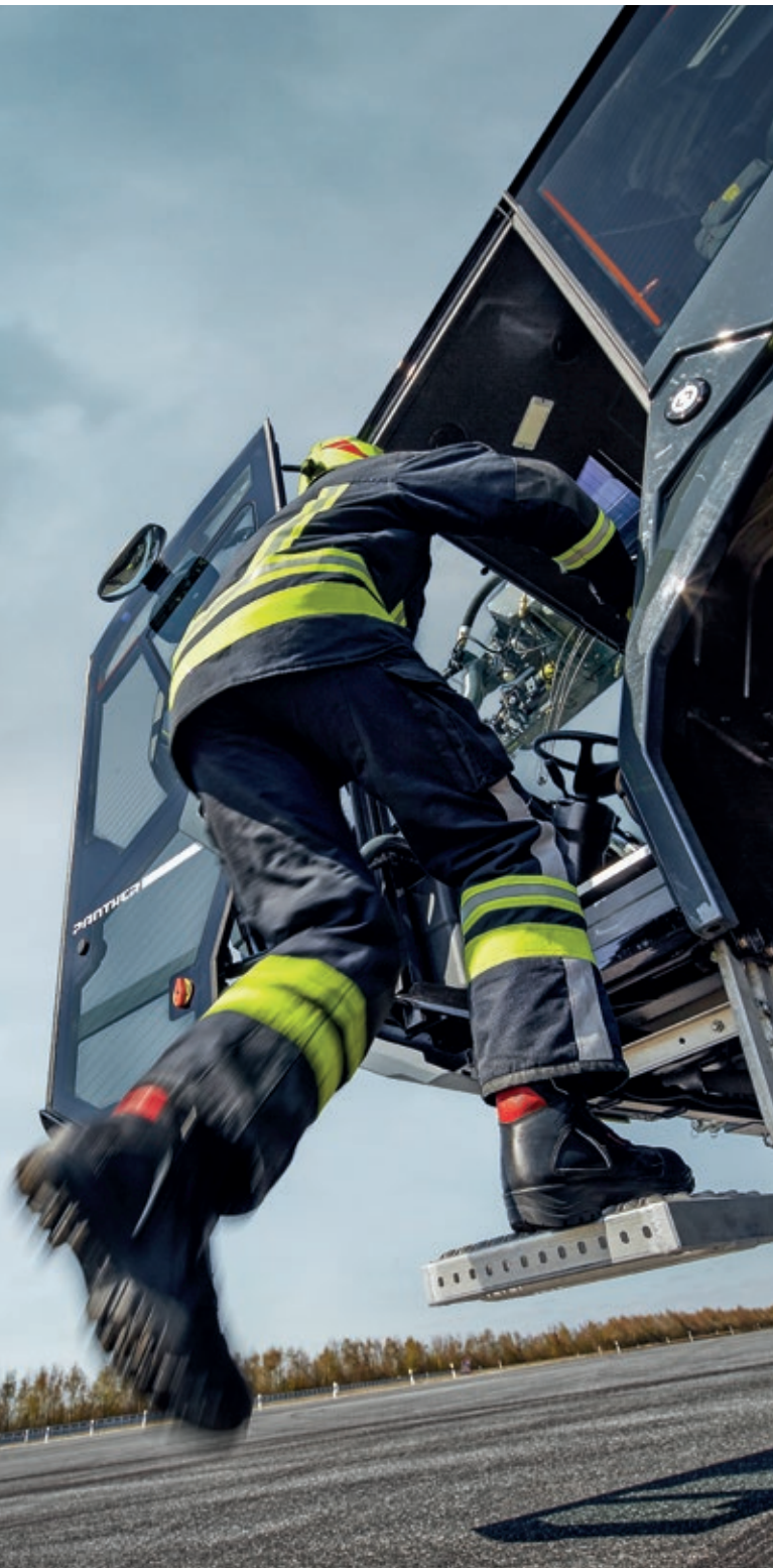
Easy access due to the swivel step
